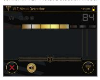
The detected object results in a signal within the grayed-out Target-ID zones.
