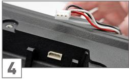
After replacing the battery, connect the plug of the new battery correctly.
