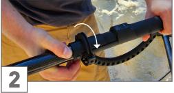
Unfold the PentaSense Rod.
