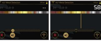
Strong signal detected in one of the active Target-ID zones. Displayed Target-ID is 58.
