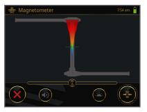
The Enhancers are not connected correctly.
