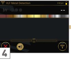
If the Ground Balance is successful, you will hear a confirmation signal (2x high-pitch beep, if Sound is enabled) and the scan screen is displayed immediately.
