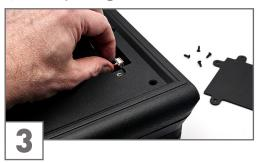
Disconnect the plug carefully. Make sure to pull the plug instead of the cable.
