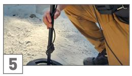
Wrap the cable tightly around the Telescopic Rod to avoid false signals while detecting.
