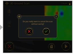
Confirm with ✓ to discard the scan and return to the Main Menu OR return to your scan procedure with X.
