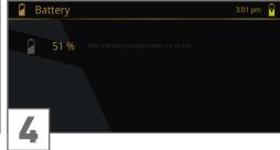
Wait until the Control Unit is charged. It can take up to 4h to fully charge the battery.
