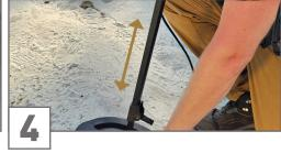
Adjust the Telescopic Rod to your body height to allow for more comfort while working with the detector. Lock the levers to fix the height.
