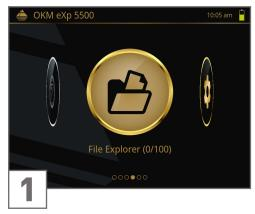
Open File Explorer. The digits in brackets show the number of scan files that are currently stored. The maximum number of scan files that can be stored is 100.
