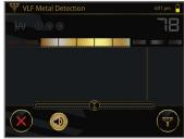
Strong signal detected in hidden Target-ID zone: The bar graph and the corresponding Target-ID are grayed out. The acoustic feedback is muted.
