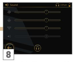
As soon as the headphones are successfully connected, you will see the Sound Settings. The symbol  $\bigcap$  in the top bar indicates that the headphones are successfully connected.
