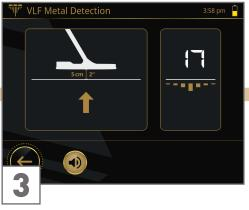
When finished, both arrows are in the target position and the 'quietest' ground value is displayed on the right. This value is saved for the current measurement.
