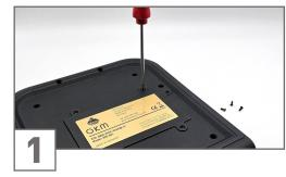
Turn the Control Unit upside down to view the Remove the battery carefully. bottom. Open the battery compartment cover by removing the 6 Torx T10 screws.
