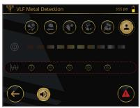
Select at least one frequency to proceed with the measurement. For more details refer to 5.7.1 Configure Measurement on page 40.
