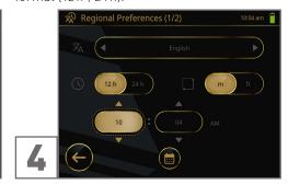
Use the arrows (up/down) to set the time (hh:mm) according to the selected format.
