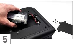
Place the battery carefully back in the compartment. Do not kink or pinch the cable.
