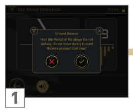
Place the coil on neutral ground (no objects underground). Hold it approx. 5 cm | 2" above the soil surface and do not move it. As soon as you are ready, start the Ground Balance with ...
