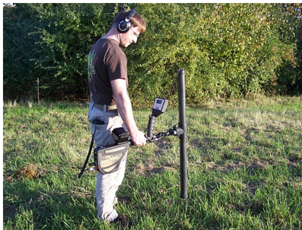
Figure 7.5: Probe should point always to the down and should not be turned
