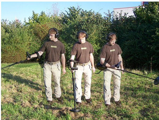
Figure 7.3: Swinging the search coil in operating mode "Metal Detector"
