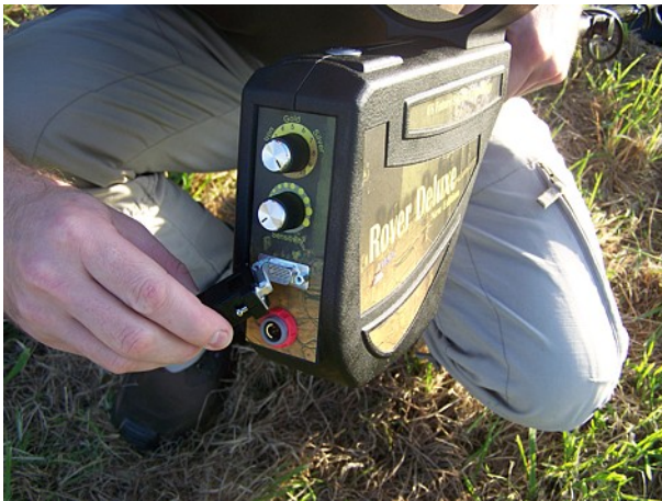
Figure 6.5: Connect control chip
