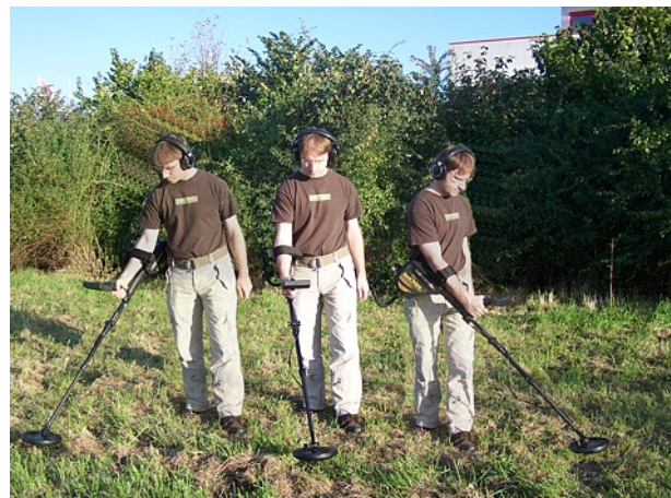
Figure 7.3: Swinging the search coil in operating mode "Metal Detector"
