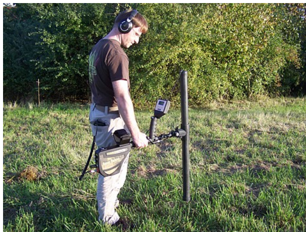
Figure 7.9: Position of the Supersensor during a measurement
