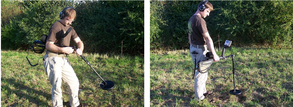
Figure 7.6: The search coil should be bent while using "Ground Scan"
