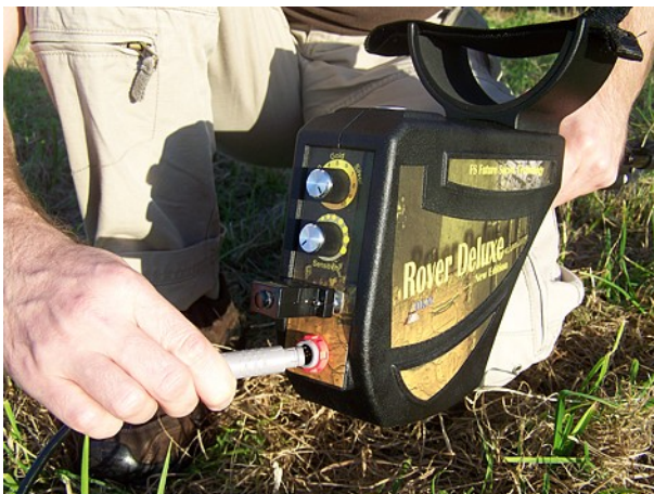
Figure 6.6: Connect power pack for power supply
