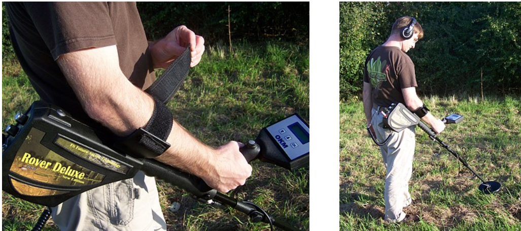
Figure 7.2: Handling the Rover Deluxe in operating mode "Metal Detector"
