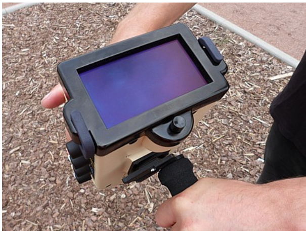
Illustration 4.6: Rotate the control unit to fasten it
