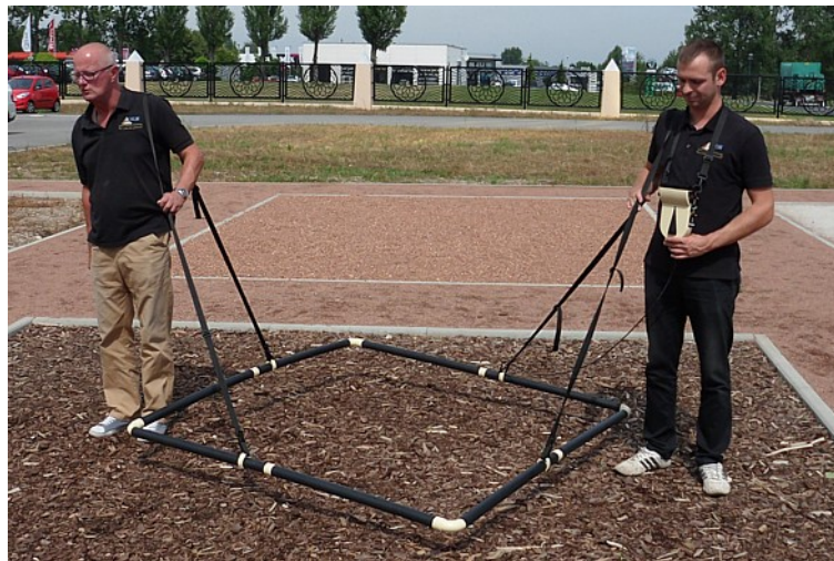
Illustration 4.20: The frame coil can also be carried by 2 people
