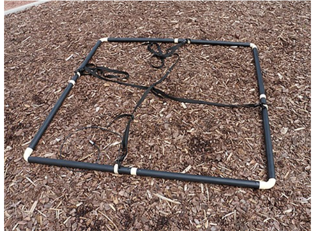
Illustration 4.17: Completely assembled frame coil
