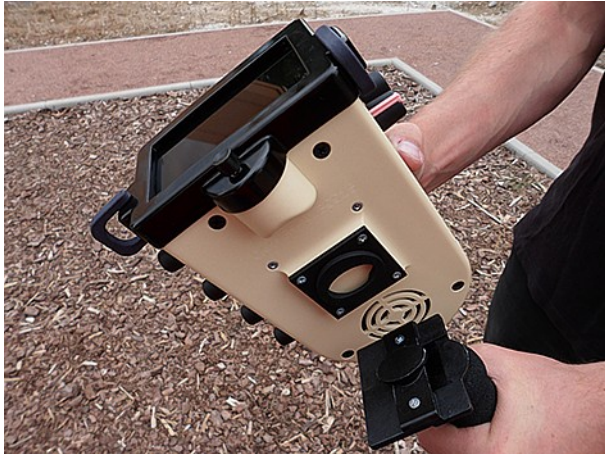
Illustration 4.4: Align bracket to control unit
