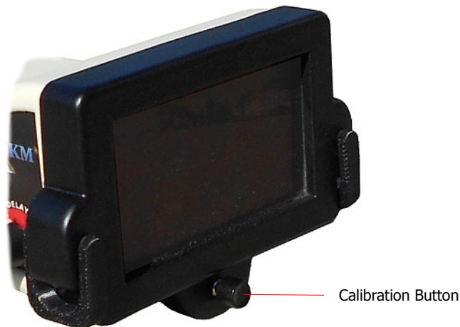
Illustration 5.11: Front of control unit
