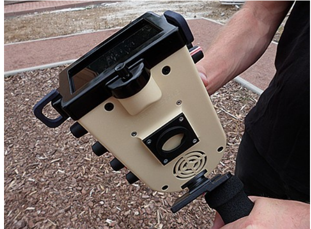
Illustration 4.5: Both brackets must connect firmly
