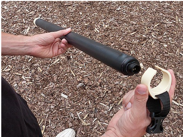
Illustration 4.12: Push belt clip over coil segment
