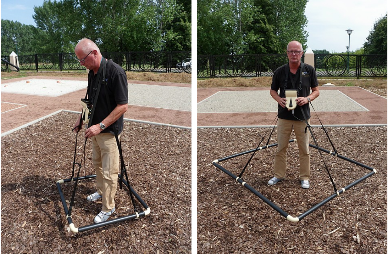
Illustration 4.19: The frame coil can be assembled in different sizes
